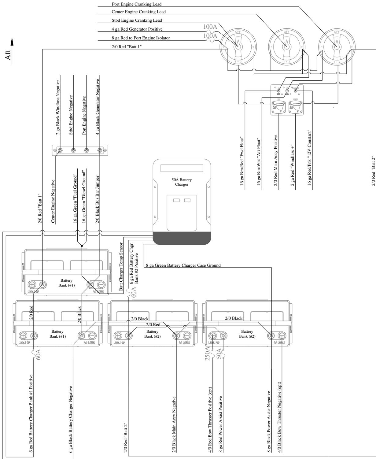
NOTE 1: 50A engine isolator fuse changes to 100A MRCB if the boat is equipped with V6 engines.
